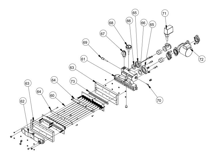
Figure 22. Heat Exchanger Components.
